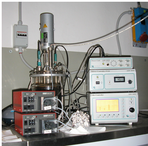
Reactor used for specialized biomass growth and biomass microscope
