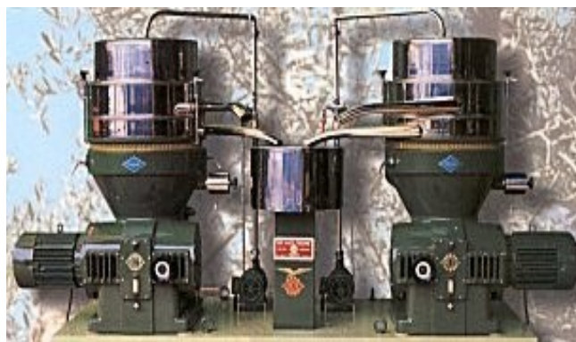
Vertical centrifugal machines (in parallel) for OMW by olive oil separation
