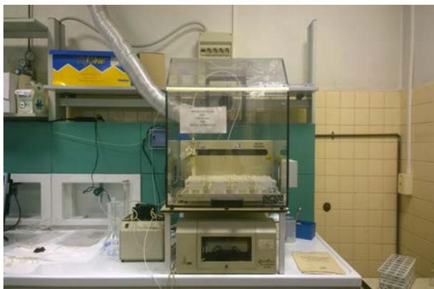
Figura 3 - ICP-MS Thermo Scientific iCAP Qc
