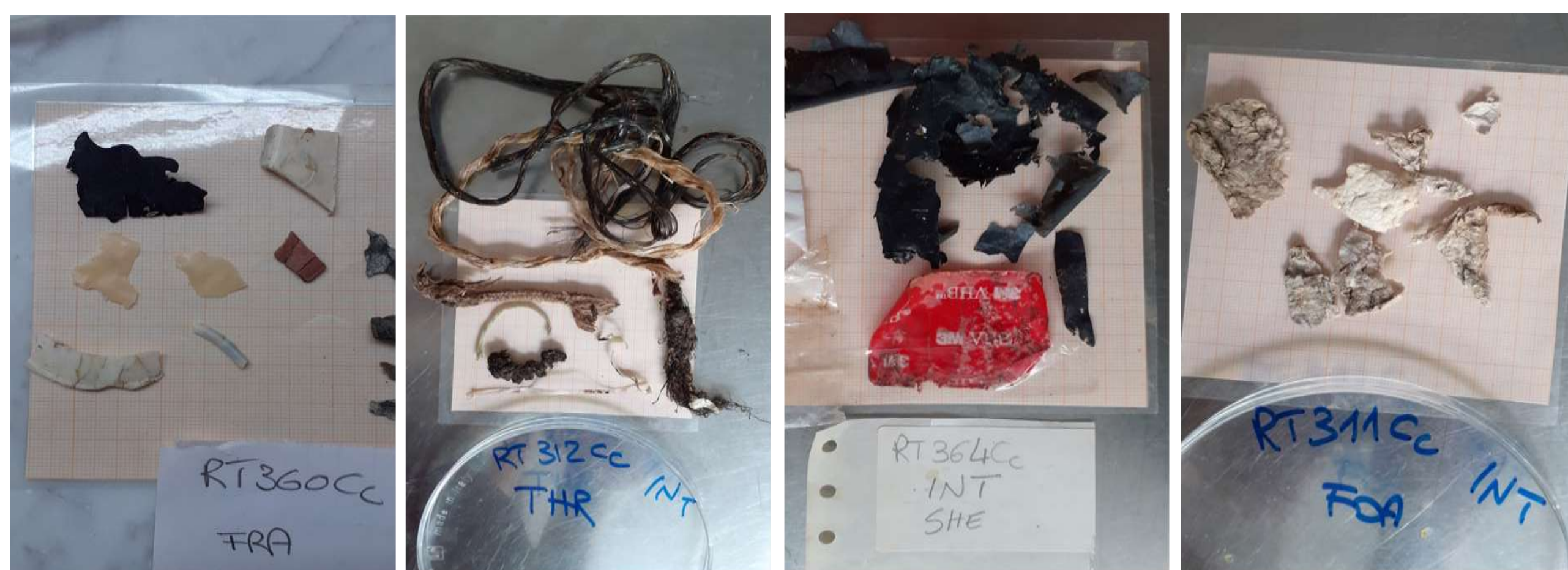
Different type of plastic categories: fragment (FRA), threadlike (THR), sheet like (SHE), foamed (FOA), other plastic like (POTH), industrial plastic pellets (INDPLA), other non plastic litter (OTHER)
