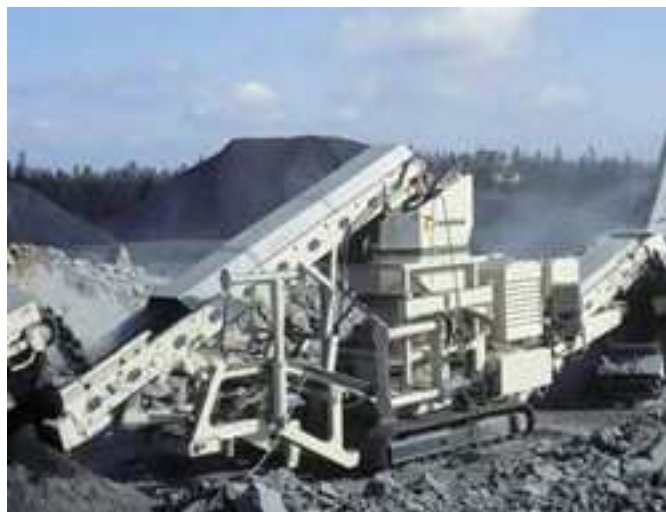
Mobile plant for secondary (SCC 3-05-020-02) and tertiary crushing (SCC 3-05-020-03)
