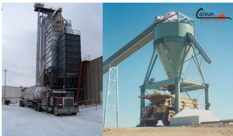
A sinistra: Bulk Loading, “Construction Sand and Gravel” SCC 3-05-025-06; a destra: Truck Load-out, “Asphalt Concrete” SCC 3-05-002-14
