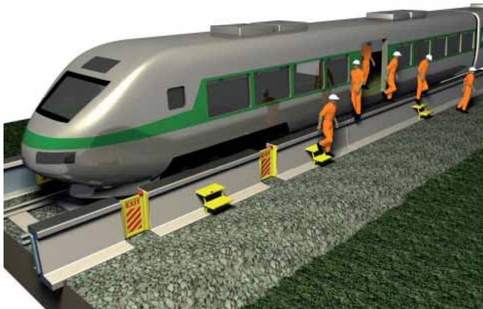
Figura 43 - Barriere basse calpestabili vicine al binario [da Probst W., “Q-city: a concept for noise mapping, ranking, hot spot detection and action planning”, 2007]
