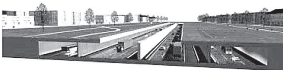
Figura 62 - Tunnel parzialmente aperto sulla A2 Leidsche Rijn – Utrecht, in Olanda [da Q-City TIP4-CT-2005-516420, Quiet City Transport DELIVERABLE 6.2 Consolidation - Action Plans – Dissemination, 2007]
