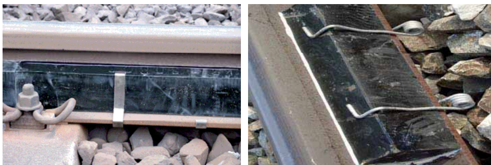
Figura 37 - Assorbitori fissati meccanicamente, particolari [da Benton D., Engineering Aspects of Rail Damper Design and Installation , 2006]
